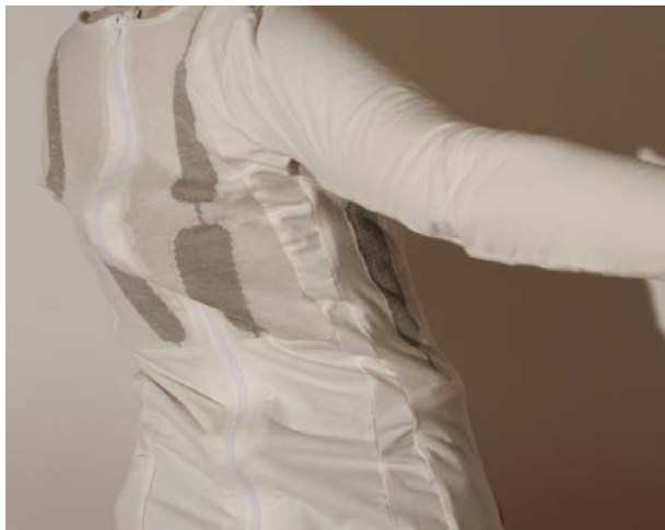
Figure 1: The shirt with sensors (the gray areas) that was part of the Vigour PSS prototype.
