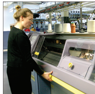
→ Jesse Asjes is setting up the Stoll knit and wear machine in the TextielMuseum TextielLab.
