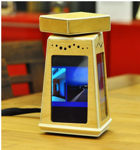
Figure 4. Photo of the 4Photos prototype with the rearranged displays, domestic aesthetic and rotatable top part.
