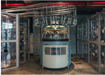
Figure 1: The fabric tube knitted on the circular knitting machine can have a combination of different patterns and shapes.
