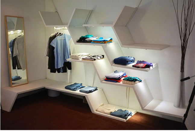
Fig. 1. Overview of the walk-in closet’s design with ceiling spots to lighten the overall environment, and shelf lights that are used to express the system’s behavior. Pressure sensors under the carpet track the user’s general location, whereas infrared sensors are able to recognize hand movements nearby each shelf.
