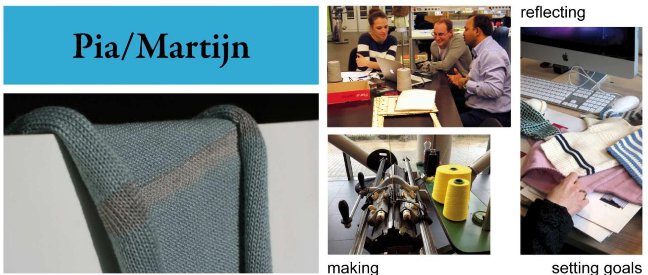
**Result 2.** Pia Maria-Laux and Martijn ten Bhömer developed a knitted fabric that can measure stretch of the fabric. In this fabric the sensor would be directly integrated, enabling the fabric to be used in regular textile garments. For example to measure body movement when integrated in
