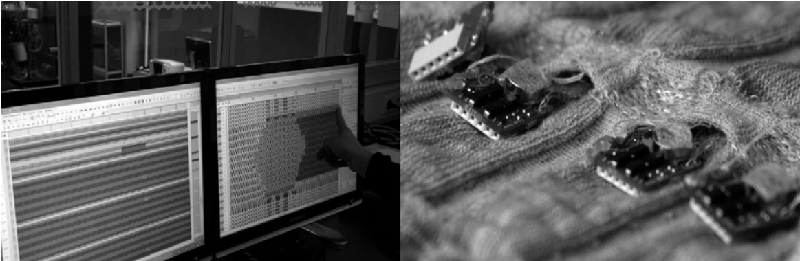
Fig. 2. Left: the computer interface to design the pockets. Right: the bottom of the pockets, showing the touch sensitive fabric, the connection lines and the electronic modules
